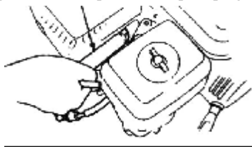
Special socket spanner for spark plug
