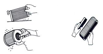
figure 3 (papery filter element)
